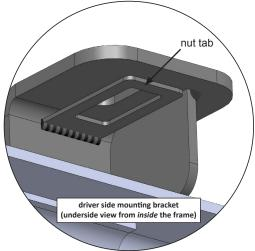
5. Fish the Bolt Leader and Spine Bolt between the opening of the frame on the inside of the frame, and out through the 17/32" hole in the frame and bracket on the outside of the frame (see illustration below).
