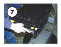
7. Put plate in location using two 9/16-12" bolts opposite corners to hold plate.
