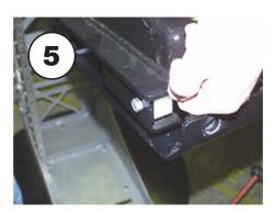
5. Install and tighten nut (self locker) x 4.
