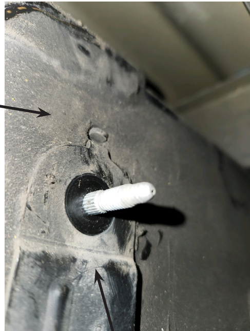
Auto level system brace/fastener
